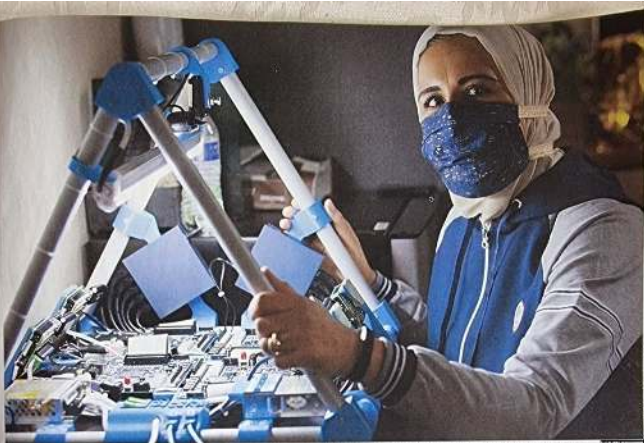
Rania Hussein, an assistant professor at the University of Washington in Seattle, is shown with the Intel Field-programmable gate array remote laboratory at the school. Students use a Web browser to test their hardware designs on the boards.
