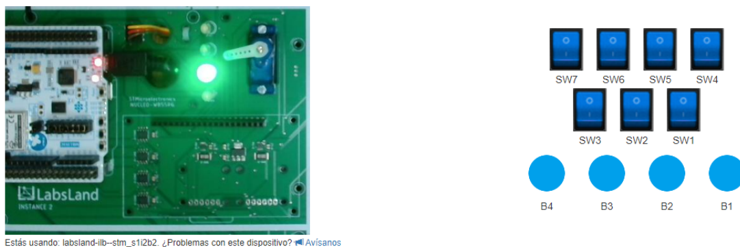
Figure 3. Main interface of the laboratory, interacting with the board.
