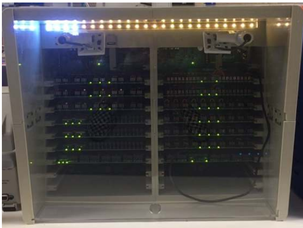
Figure 5.2: The Hive node performing automated tests. It has a yellow/orange color most of the LEDs except for 4 in this case that indicate that the board under test is the number 4.
