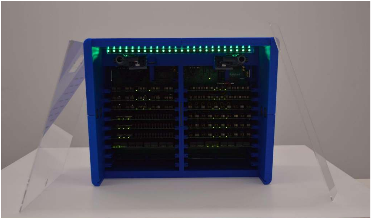
Figure 2.9: Hive node with the main and secondary methacrylate covers detached. (Supported on the sides).
