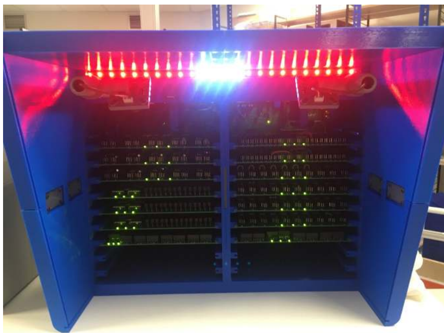
Figure 5.4: Hive node displaying a connection error to the server (4 white LEDs in the middle, all the rest are red).
