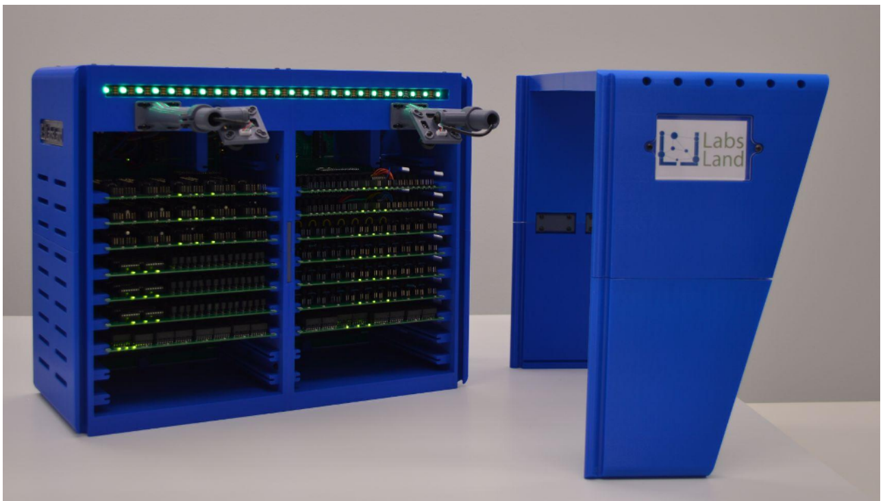
Figure 2.8: Hive node with the trapezoid detached.
