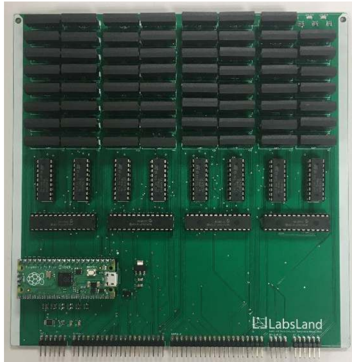
Figure 3.16: Oscilloscope and PSU board
