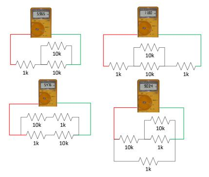
Figure 10. Serial and parallel combinations
