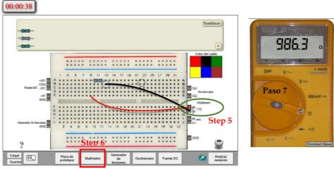
Figure 7. Measuring  $1k\Omega$  resistance with the multimeter
