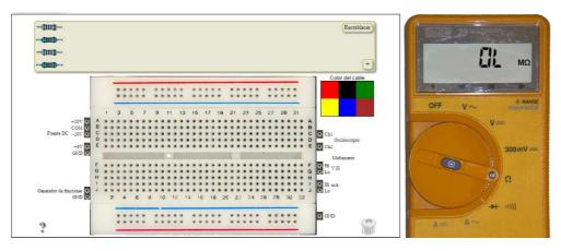
Figure 1. Breadboard and multimeter at VISIR remote Lab
