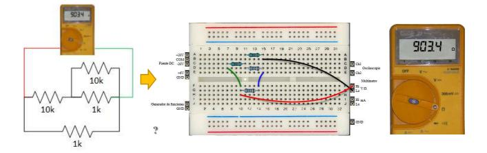
Figure 12. Example of serial and parallel combination
